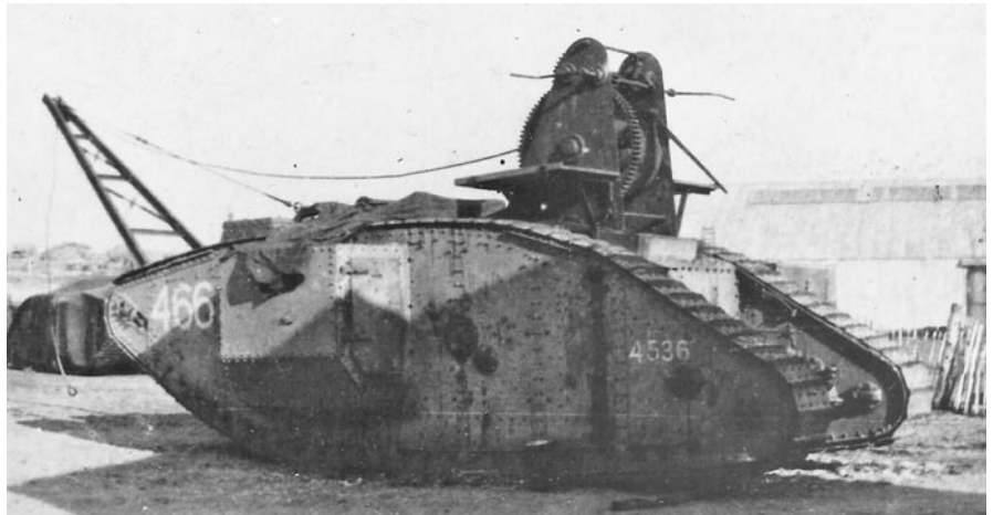
Il Salvage Vehicle basato sullo scafo del carro armato Mark IV ( https://tankmuseum.org/article/experimental-tanks-part-two )
